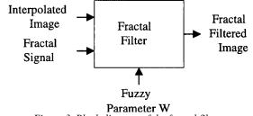
Figure 3. Block diagram of the fractal filter.
